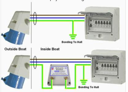
mains electricity supply enters the vessel, or close to the fuseboard.
