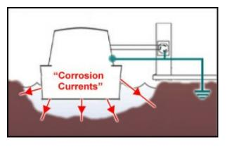
Although corrosion currents can be quite small, over a period of months, your boat could shed many many kilograms of its hull, leading to pitting, and even holing.
