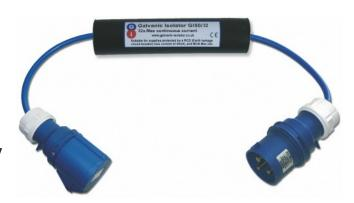
It is only necessary to use a galvanic isolator when you are connected to shore (mains) power. It is not necessary when you are using a generator or other power source that is not connected to Earth. Ensure that no ground connections on the vessel bypass the Galvanic isolator.
