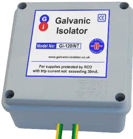
The Gi120/NT Galvanic Isolator is intended to prevent galvanic and stray currents from finding a circulating path through the earthing connection of a shore supply.
